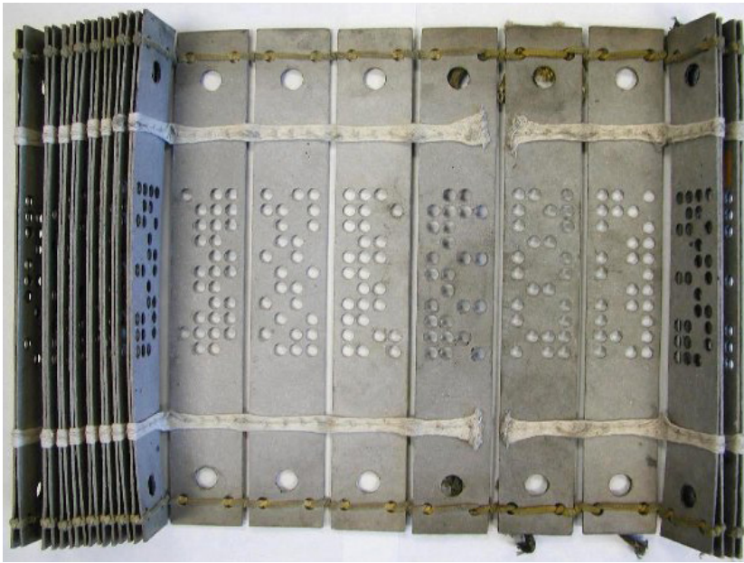
The binary principle embodied in the punched-card operation of the Jacquard loom was inspiration for the data processing machines to come, and the use of replaceable punched cards to control a sequence of operations marked an important step in the history of computing hardware. Courtesy of Douglas W. Jones, University of Iowa.
