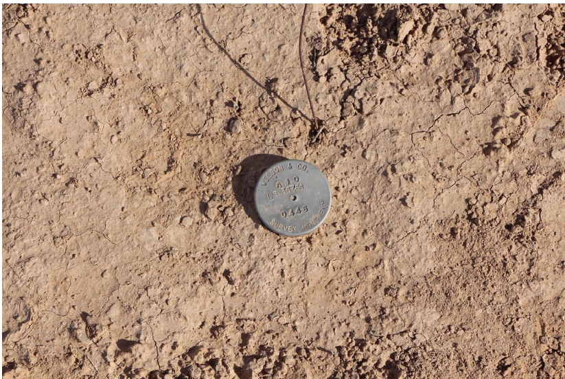
US Customs and Border Protection survey monument for surveillance tower on the Tohono O’odham Nation. Photograph by the authors.
